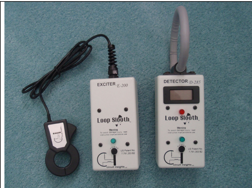
Figure 4. Left: D-200 Exciter, Right: D-285 Detector with Rogowski coil tucked in retainer at top of module.
